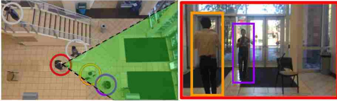
Figure 1.4: A pair of top- (left) and egocentric (right) views. Self identification is to identify the egocentric camera holder (shown in red). Human re-identification is to identify people visible in the egocentric video, in the content of the top-view video (orange and purple).
